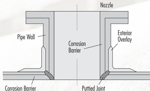
The illustration above represents an old method of attaching nozzles to pipe by filling the interior joint with putty. This nozzle is very susceptible to corrosive attack because vibration, turbulence and flexing at this point will erode the putty out of the joint area, causing the system to fail.
